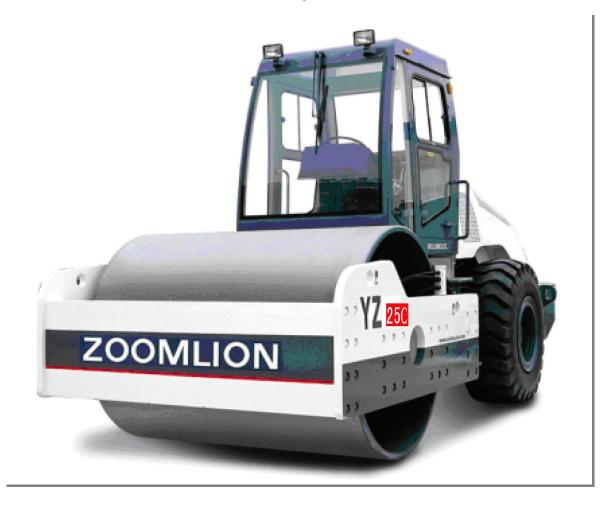
**YZ25C** vibratory roller, as heavy-duty self-propelled roller, is used for high-quality earth compaction in large project. It's suitable for all kinds of foundation and compaction and widely used in high-level road, railway, airport, seaport, dam, surface mine etc.
